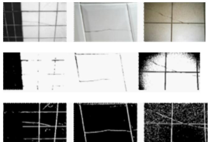
Figure 2. Example of a pre-processing: (up) Original image, (middle) Simple binarization, and (down) performed pre-processing on the original image.
