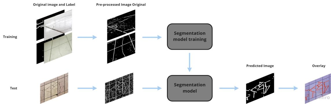
Figure 1. Architecture for crack segmentation.
