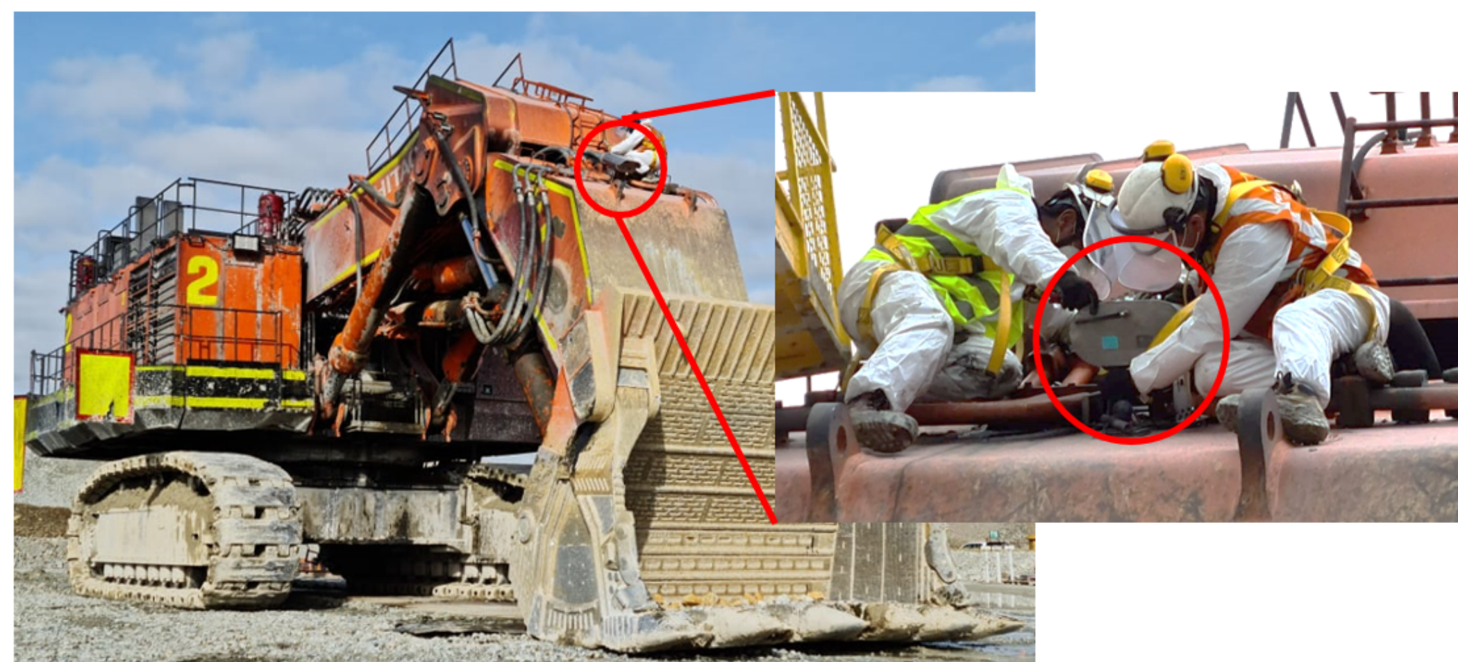
Figure 1: Installation of thermal camera in metal chassis in excavator
