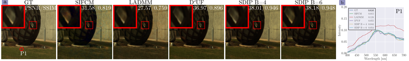
Figure 4. a) RGB visualization comparison with state-of-the-art methods, SIFCM [29], LADMM-NET [26], D 2 UF [14], and the proposed method SDIP for B = \{4, 6\} on the ICVL dataset, upper-right numbers show the PSNR and SSIM scores. b) Spectral reflectance and SAM score comparison of a random point compared to the reference signature.
