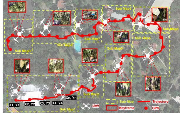
Figure 2. General diagram for the sub-maps creation and keyframes storage. The flight trajectory is shown in red, circles express GPS coordinates, keyframes are in red squares, and sub-maps are in yellow rectangles.
