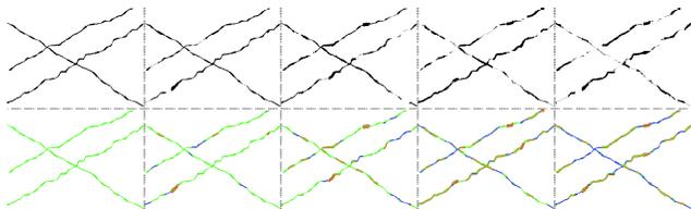
Figure 2. Examples of label noise levels 0 to 4 (see Table 2). The second row shows: Green) Crack pixels; Blue) Crack pixels mislabeled as background; Red) Background pixels mislabeled as crack.
