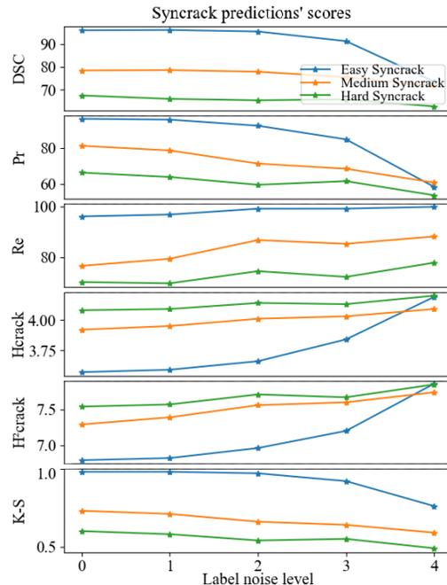
Figure 3. Prediction scores obtained in the validation splits of the Syncrack’s 3 difficulty levels evaluating with accurate annotations.
