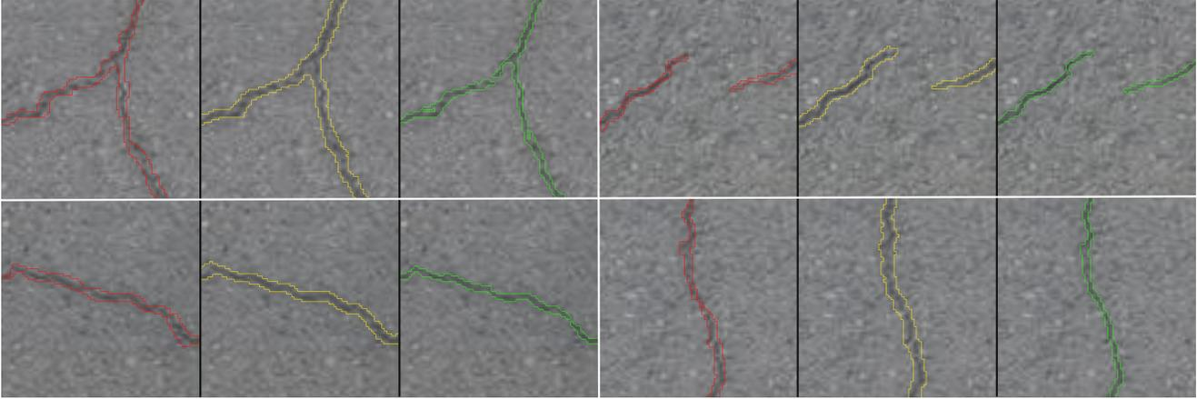
Figure 4. Examples of crack segmentation borders. The red line is the border of the manual annotation, the yellow line is the border of the prediction obtained by training on CFD, and the green line is the border of the prediction obtained by training on Syncrack hard.
