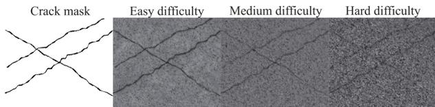
Figure 1. Example of Syncrack-generated images. The leftmost image is a synthetically generated crack shape. The rest of the images are synthetically generated backgrounds with the same inserted crack.
