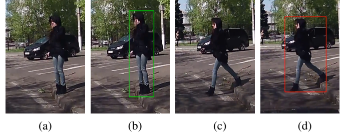
Figure 4. Results of intention prediction (a) Pedestrian is standing on the curb (b) The green bounding box around the pedestrian generated by our network shows that the pedestrian is not crossing the road (c) The pedestrian is intending to cross the road (d) The red bounding box around the pedestrian signifies the crossing intention of the pedestrian.
